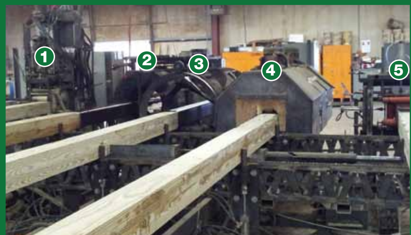
This 5 - Cell automated application work center can be used by two (2) warehouse employees and can work on 5 posts at a time.
